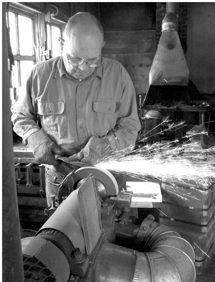
Vic Hargas rough grinding a hand forged Ruana blade on a stone wheel.
